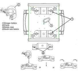
Regardless of the rigging option you choose for your SPOT LED, always be sure to secure your fixture with a safety cable. The fixture provides a built-in rigging point for a safety cable on the hanging bracket as illustrated above. Be sure to only use the designated rigging point for the safety cable and never secure a safety cable to a carrying handle.
