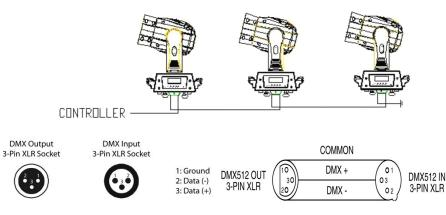
For installations where the DMX cable has to run a long distance or is in an electrically noisy environment, such as in a discotheque, it is recommended to use a DMX terminator. This helps in preventing corruption of the digital control signal by electrical noise. The DMX terminator is simply an XLR plug with a 120  $\Omega$  resistor connected between pins 2 and 3, which is then plugged into the output XLR socket of the last fixture in the chain. Please see illustrations below.
